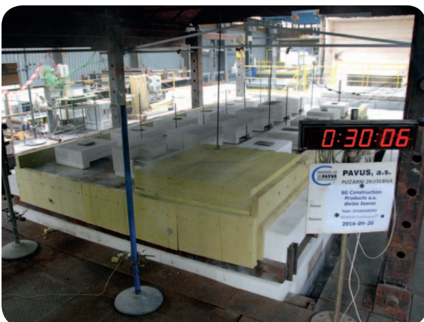
Fig. 11 Sample after 30 minutes – fire protection system Isover FireProtect® fulfils its function for 100 %, roof is without any deformation (bending stress, the same as would be under cold conditions)
